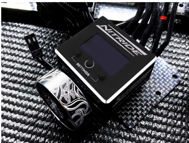
Example of NITRIDE installation into on-road car using the fan for use with the motor 4,5T on asphalt
